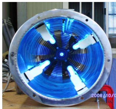
System of air disinfection with a forced ventilation tunnel for high flow rate
